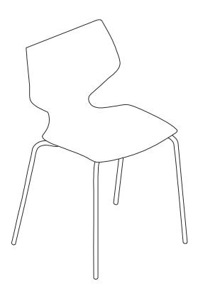
Attach 1 x seat (A) to 1 x legs (B) and secure with 4 x bolt (C) and 4 x washer & nut. Tighten with an allen key (D).
